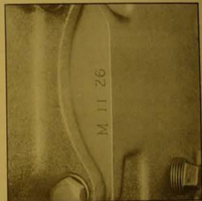
Fig. 6—Conventional transmission unit number located on rear face of case in the upper right corner. O.D. unit, same identification.
