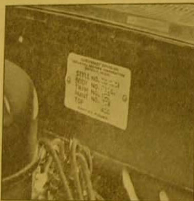
Fig. 4—Body style, body number, trim type and paint combination located on the dash panel directly above the distributor.
